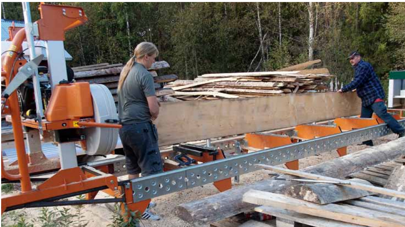
• The sawmill LumberMate Pro can without problem take logs that are 70 centimetre in diameter.
