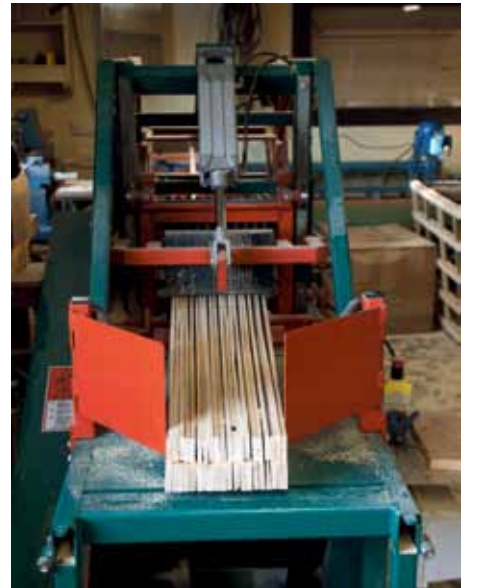
Eight millimetres. That's how thin the boards are, which are sawn with little sawdust losses and perfect dimensions.
