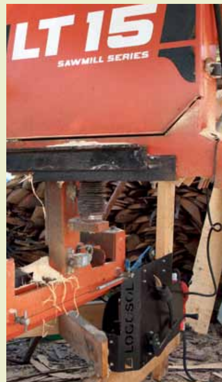
The Logosol friction feeder works perfectly on LT15 sawmill.
