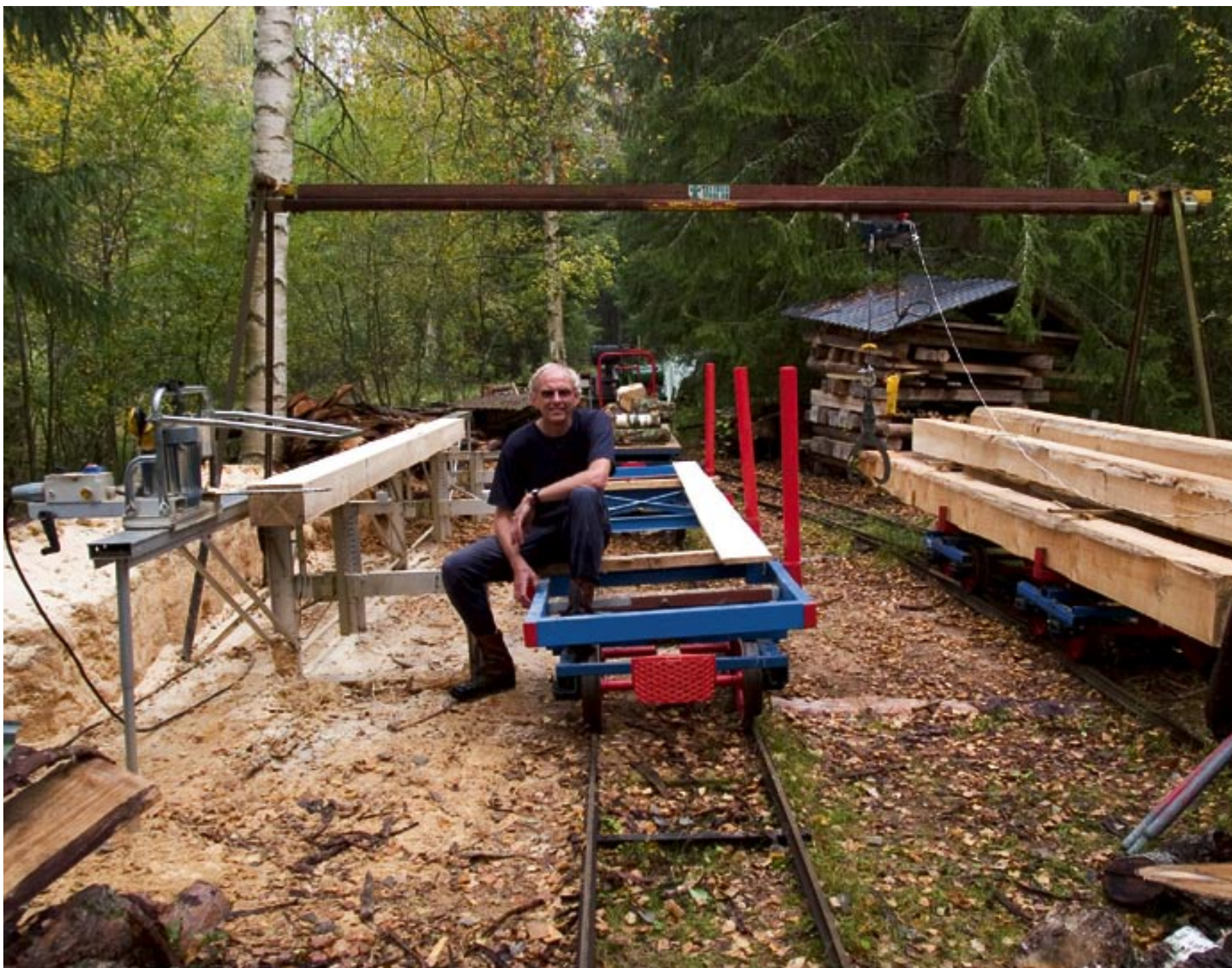
Bo Malmberg works as a production technology manager at Electrolux in Motala. Due to this, it is not surprising that the logistics around the sawmill is well thought out. The logs arrive on the track to the right. Then, they are lifted onto the Logosol Sawmill with the help of the electric gantry crane, and finally boards and planks are placed on the wagon to the left and transported to be seasoned.
