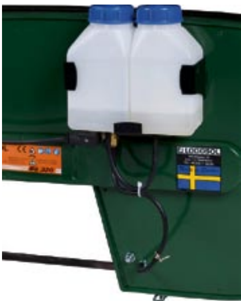
The new water cooling with automatic shut-off: Now also on Logosol's bandsaw.
