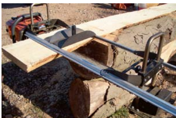
Rest the assembled mill on the reference plank, and open the throttle to full revs
