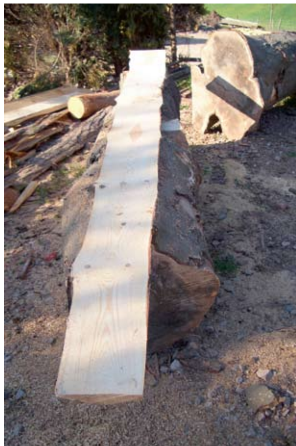
After trimming off any projections, the plank is screwed securely in place.
