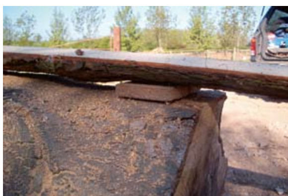
Use packing pieces between the plank and the log to prevent it from twisting.
