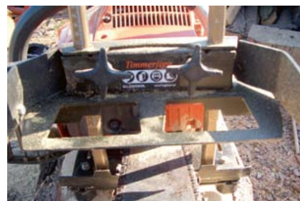
Two knobs on the Timberjig allow you to set the height against the scale.
