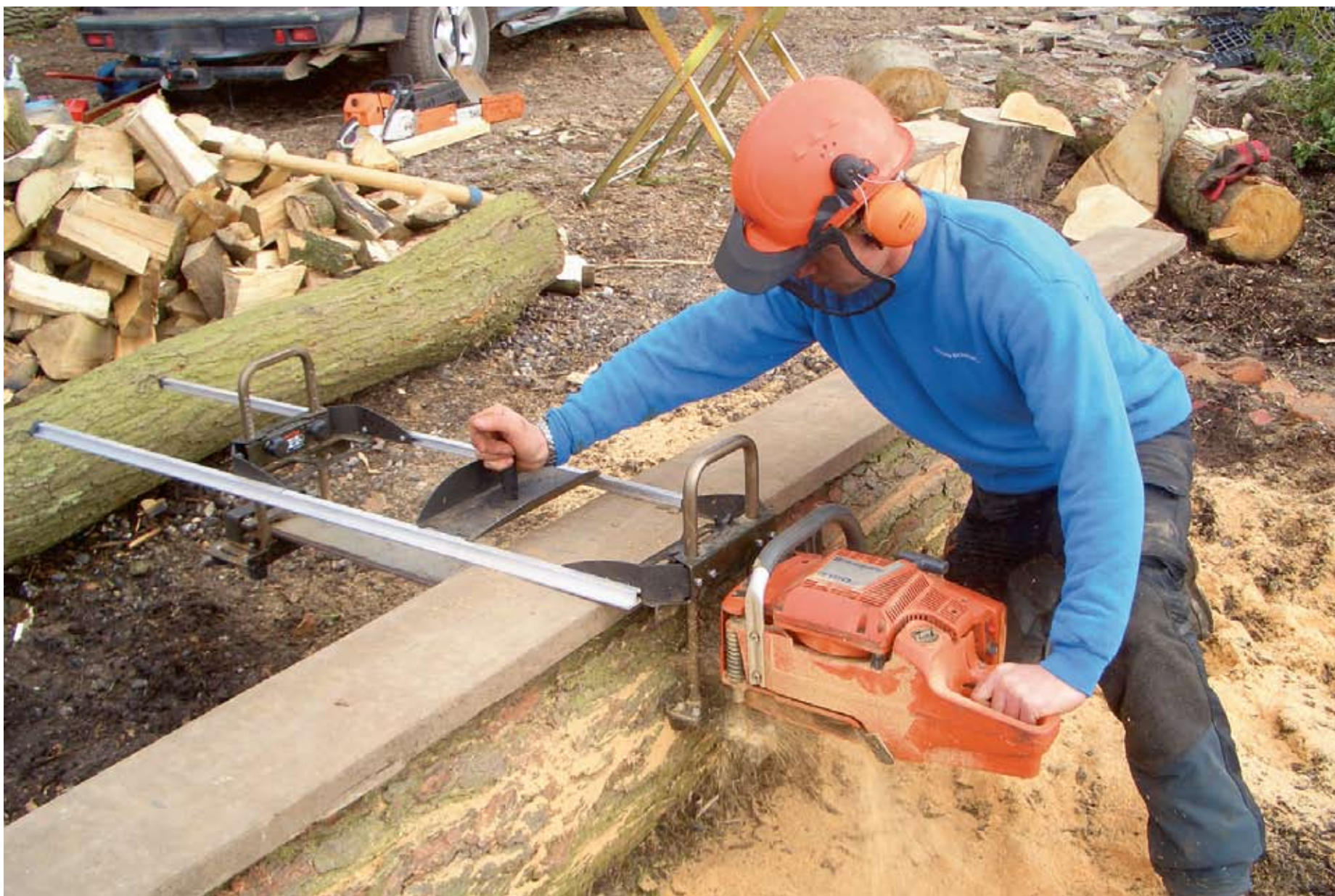
With the Logosol LSG you can saw giant logs, Richard Dunmore explain how it works.
