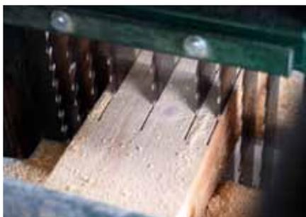
*Specially designed carbide tipped blades give one to two days of full production before sharpening.*
