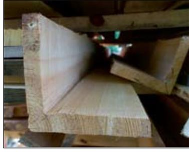
Wedge-shaped and wide siding boards are sought-after products.
