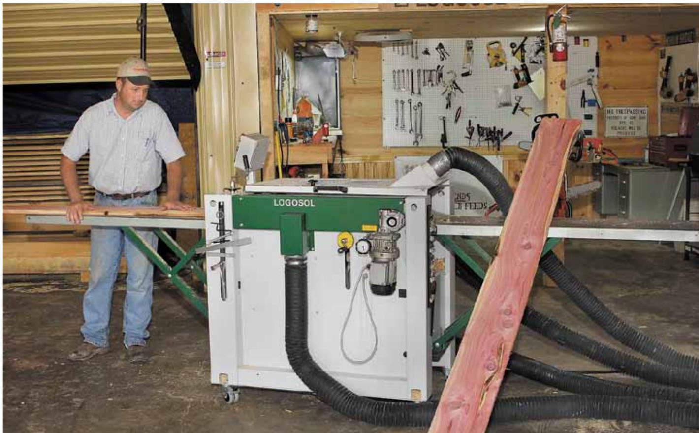
*Rusty with his PH260 Model 3. Notice the setup tools attached to the front of the planer on a magnetic strip. The kiln Rusty built is behind him.*
