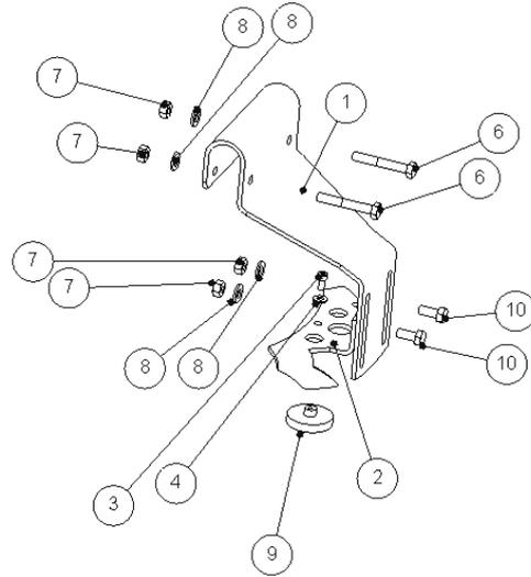
Components, bar nose steering for petrol chainsaw:
