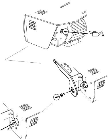
Lubrication of both sides of the friction clutch and the spindle. After maintenance is done, the neutral mode of the feed unit must be adjusted (see p.24)
