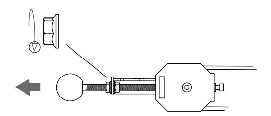
Finish the adjustment by tightening the counter nut.
