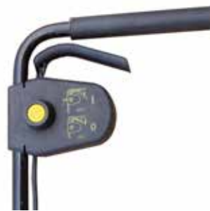
The bandsaw's start control with "dead man's handle".
