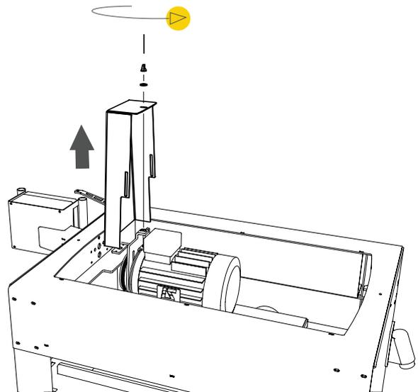
**2** Refit the wing nut and the washer. These are necessary for carrying out the adjustment.
