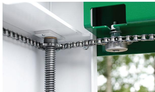
*The chain transmission should run easily! In the photo you can also see the chain tensioner.*
