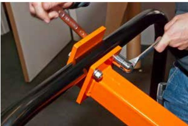
8. Fit the sliding rail. Start by fitting it to the tube arch using **two M10x80 + M10 lock nuts and M10 washers** on the side where the nuts is.
