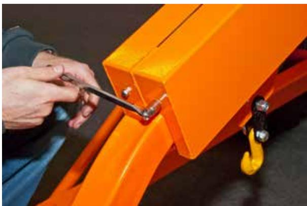
12. Fit the cover over the sliding rail with the opening for the tube arch facing the rear of the trailer. Secure the cover with **four M6x16** including **M6 washers**.
