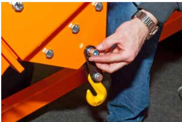
11. Fit the link plates and the lifting hook to the sliding rail, using **two M10x40** including **M10 lock nuts** and **M10 washers**.
