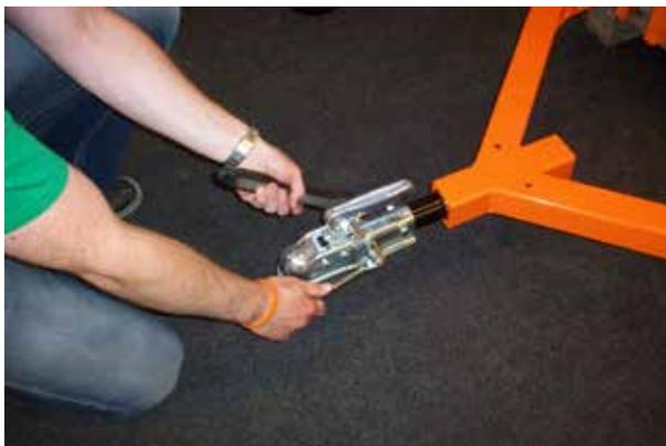
3. Install the black tube spacer on the trailer hitch axle and then fit the ball coupling using **two M10x55 + M10 lock nuts**.
