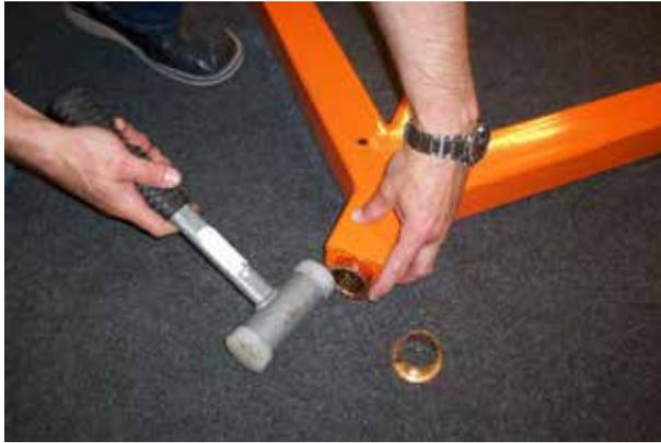
1. Start by fitting the two bushings for the trailer hitch axle in the front part of the frame, one on each side. Use a rubber mallet and tap them gently into place, as seen in the picture.
