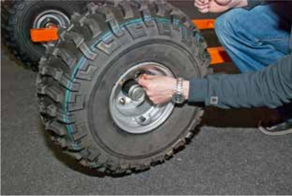
5. Fit the wheels using the included **M12 wheel nuts**. Note that the tapered side of the nut should be facing the wheel rim, in order to centre the wheel on the hub.
