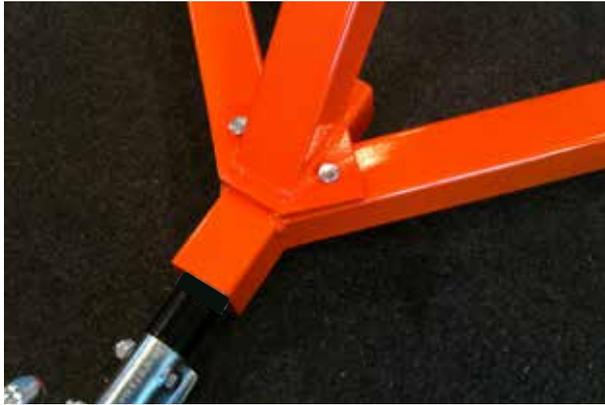
9. Fit the sliding rail front mount to the frame using **two M10x85 + M10 lock nuts** and **M10 washers** on the side where the nuts is.
