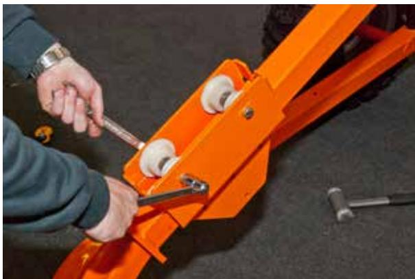
10. Assemble the side pieces, including rollers, using **two M10x100, two M10 lock nuts, two M10 washers** and **three M10x25, three M10 lock nuts** and **three M10 brickor**.
