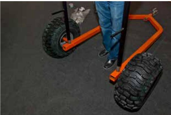
6. Press the tube arch onto the shaft stubs at the rear of the frame.
