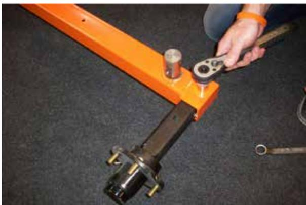
4. Fit the wheel hubs by inserting them into the square-shaped holes at the rear of the frame, as seen in the picture. Secure them with one **M12x60 + M12 washer** and one **M12 lock nut** (the nut is placed in a hexagonal hole on the lower side of frame). Tighten firmly.
