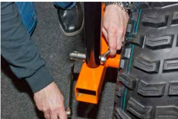
7. Secure the tube arch with **two M10x60 + M10 lock nuts and M10 washers**.
