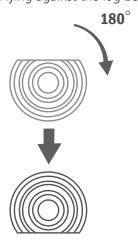
Turn the log through 180° so that the freshly sawn side faces towards the log bed.
