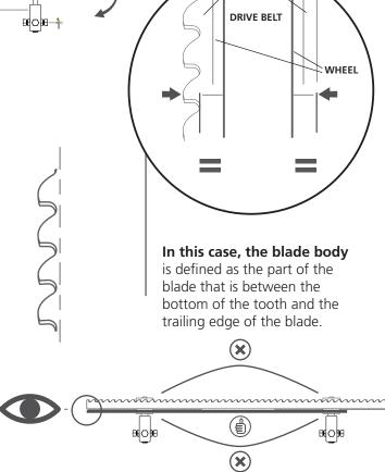
If the blade curves in the sawing direction, the blade is too far forward on the wheels. If it curves in the other direction, it is too far back.
