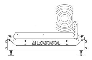
Turn the log through 90° so that one of the freshly sawn sides rests against the log supports, then clamp the log in position.
