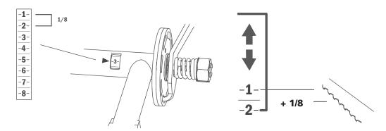
There is an opening on the shaft of the crank where a number can be seen. This is numbered in eight steps, each step being equivalent to one-eighth of an inch. **TIP:** You must always compensate for the thickness of the saw blade, i.e. 1/8", when sawing a board on the top side of the saw blade. There is never any need to compensate for the piece of wood on the underside of the blade. This has the dimension found on the absolute height gauge.
