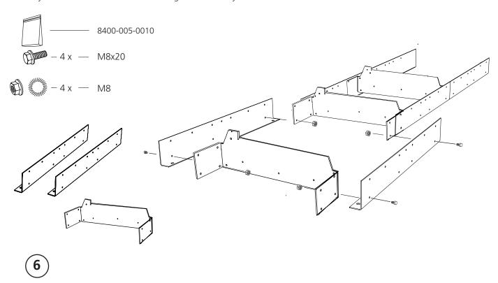
Assemble the rail sections with the log bed. Note that these must only be fitted in the lower hole and tightened loosely.
