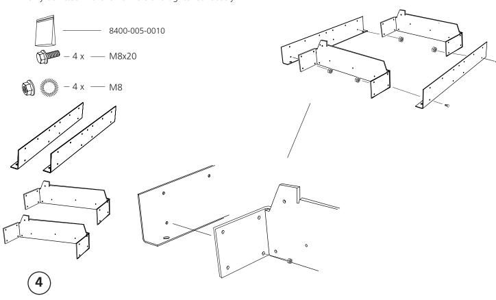
Assemble the rail sections with the log bed. Note that these must only be fitted in the lower hole and tightened loosely.
