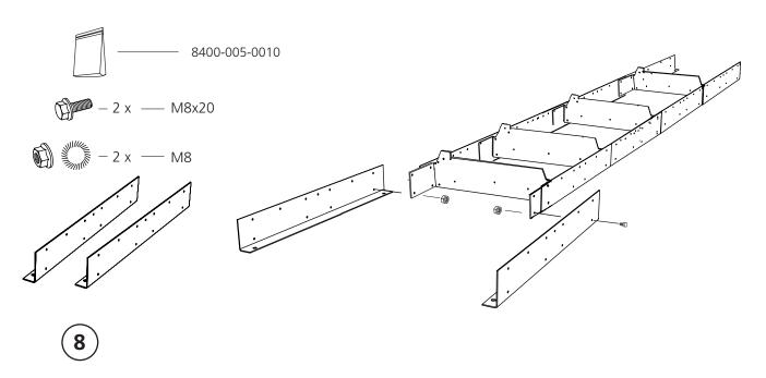
Fit the inner end cap plates to the outer ones. Note that the two shock absorbers must be mounted in the upper corners.
