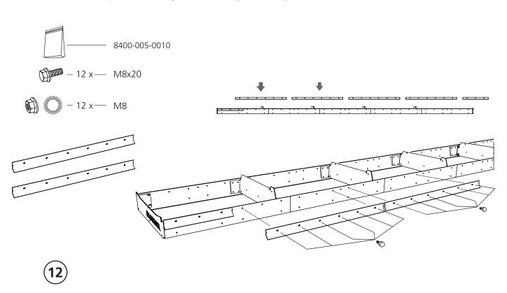
Fit the last three pieces of rail. Note that the short piece must be located at the end of the rail. Tighten the screw joint loosely.
