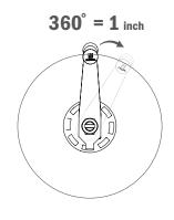
The crank locking mechanism is divided into eight positions on a single rotation. Each position is equivalent to movement of the saw head by an eighth of an inch, and a full revolution is equivalent to 1 inch. A 16-step dividing plate is available as an accessory.
