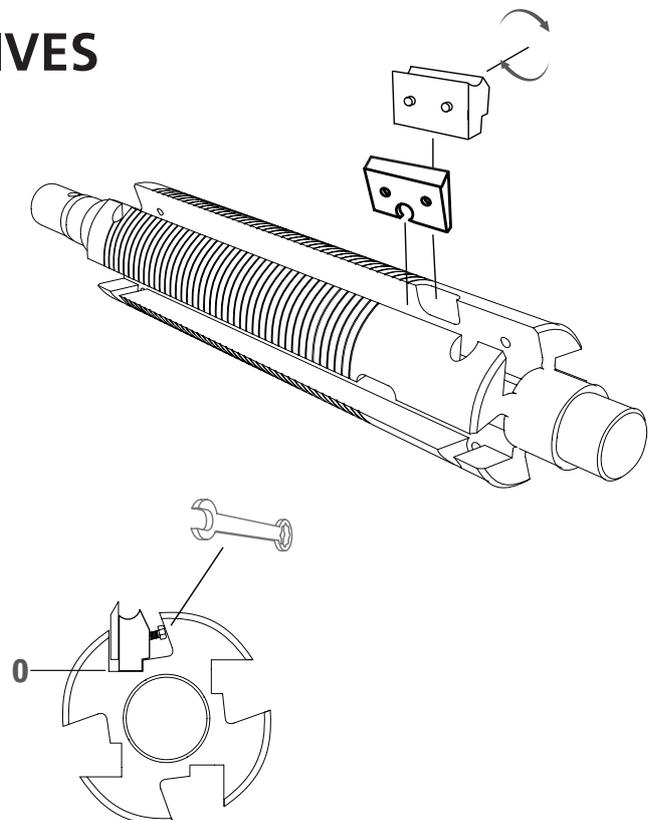
Secure the knife by firmly unscrewing the locking screw on the back of the wedge.
