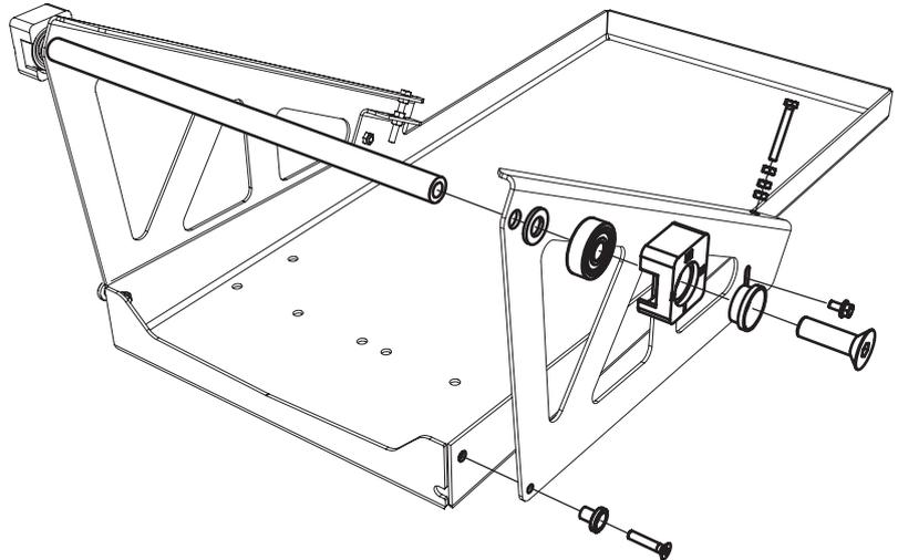
If the angle adjustment blocks aren't used, the outfeed table is assembled in the same way as the infeed table according to section 3. Then the screws and washers below are also used, these will otherwise be left over.
