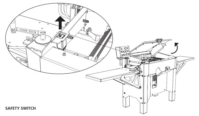
The planer is equipped with a safety switch, which is located at the front left corner of the lid. The safety switch cuts the power to all motors if the lid is opened during operation or if a work piece, which is thicker than the maximum depth of cut of the horizontal cutter, is inserted.
