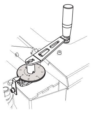
• Do not adjust the chain tensioning while raising or lowering the planer table, as incorrect tensioning can cause the chain to disengage.
