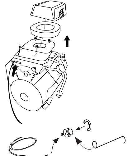
Fit the throttle link on the cable retainer, then lock the assembly into position using the lock washer.
